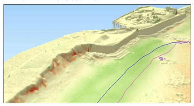
Figure 9.6: 3D view of erosion along the beach crest (reds) between 2014 and 2016. © HES.
