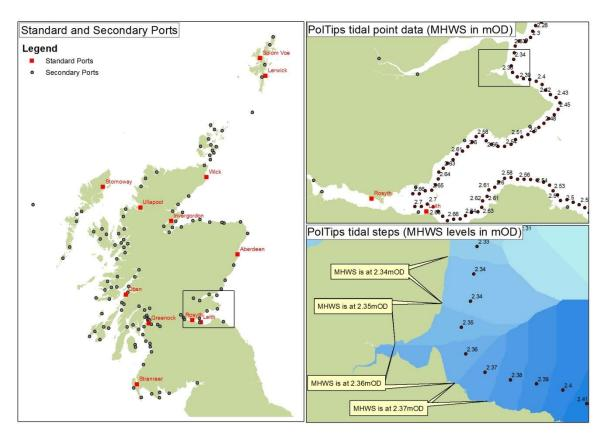
Figure 4.6: Location of Standard and Secondary Ports in Scotland, POLTIPS point data using the Coastal Flood Boundary chainage and the POLTIPS tidal steps in detail.
