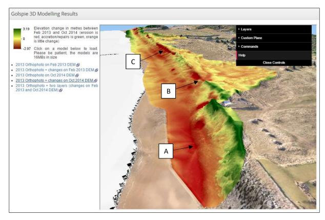
Figure 9.2 three-dimensional model of coastal changes at Golspie Links (looking south). Erosion / surface lowering shown in reds, little change in Yellows and Gains / Accretion / Repairs shown in green. See text for further description. Backdrop imagery provided by CASL © SNH.
