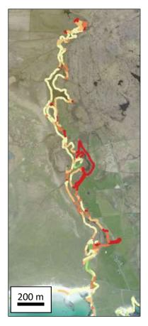
Figure 4.4: Coastal change analysis along a narrow estuary in Tiree showing the problem when the Normal Tidal Limit extends far inland. Shades of red indicate erosion, shades of green accretion. Yellow is no change. Bing Maps used for backdrop photography.
